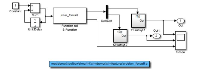
The first function-call subsystem provides a sine wave output. The second function-call subsystem is a simple feedback loop containing a Unit Delay block.
